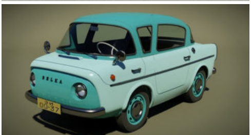
BJELKA U.S.S.R. 1956 4-seater. 2-cyl. horizontally opposed o.h.v. engine, air-cooled, at rear. Displacement 500 c.c. Max. b.h.p. 20, 4 speeds. Max. speed approx. 60 m.p.h.
