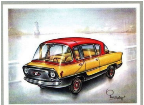
BJELKA U.S.S.R. 1956 4-seater. 2-cyl. horizontally opposed o.h.v. engine, air-cooled, at rear. Displacement 500 c.c. Max. b.h.p. 20, 4 speeds. Max. speed approx. 60 m.p.h.
