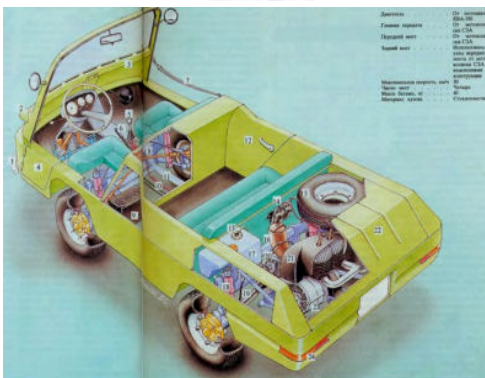
BJELKA U.S.S.R. 1956 4-seater. 2-cyl. horizontally opposed o.h.v. engine, air-cooled, at rear. Displacement 500 c.c. Max. b.h.p. 20, 4 speeds. Max. speed approx. 60 m.p.h.
