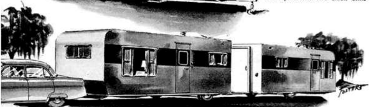
Left, a 41-foot Liberty like the one used by the author and family. It has a vented attic for better insulation. Below, the Overland Twin Liner—a 50-foot trailer that splits into two small units
