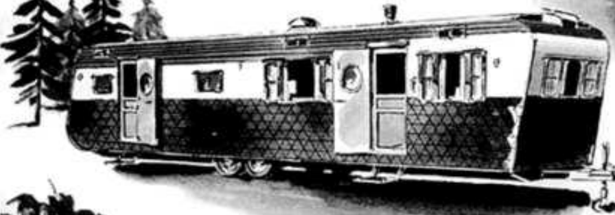
Above, Spartan uses airplane methods to build a strong, streamlined trailer with large picture windows front and rear. The sides are riveted aluminum
